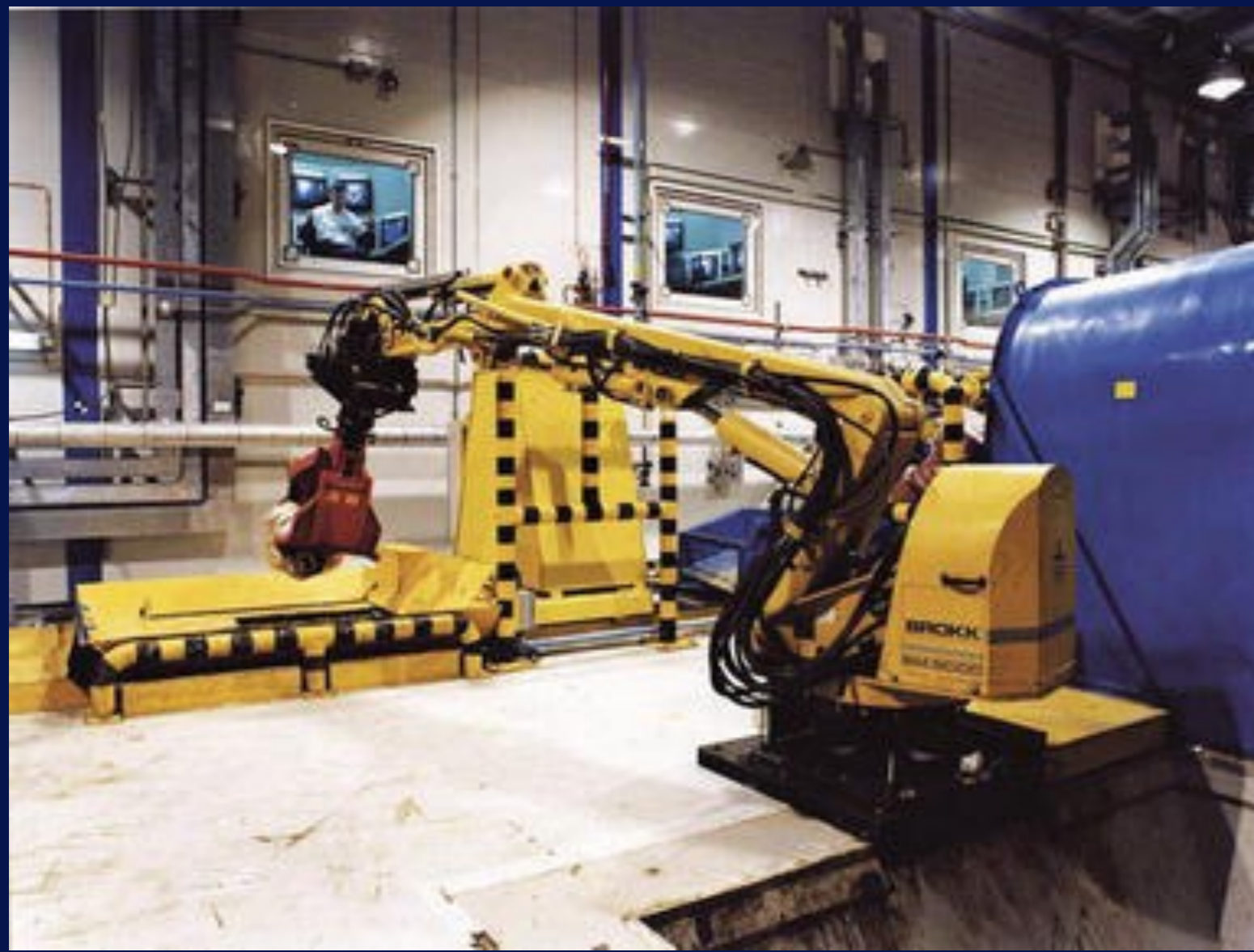
Figure 1. A BROKK robot controlled by a human operator at Sellafield, UK [1]
